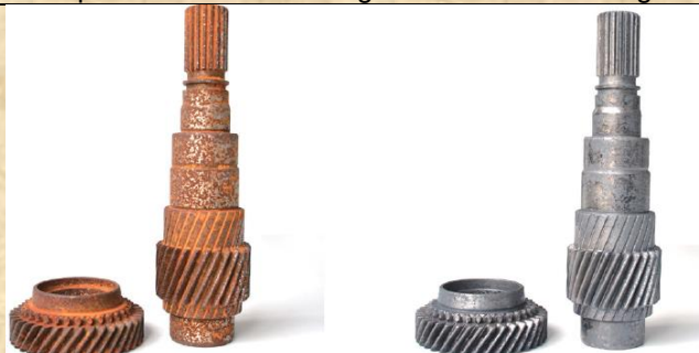
Sample: propeller gear shaft Base material: 40Cr Laser Eraser: Standard Type Erasing Efficiency: 1400mm 2 /s Erasing Effects: surface undamaged and no rust left behind
