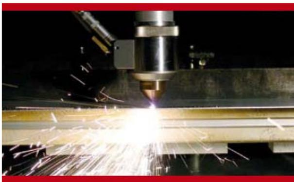
Apart from cutting in the single mode in order to create kerfs with a cut width of a few  $\mu\text{m}$ , the processing head can also be deployed in alternative optical configurations for plastic welding with foci in the mm range. For custom applications, process-supporting modules are available, such as cutting and shielding gas nozzles for welding.
