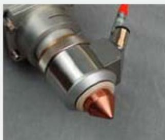
Cutting nozzle with capacitive
